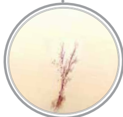
Image: electrical tree
