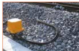
These cables connect trackside counting points which determine train presence, direction of travel, length, number of wagons and integrity.
